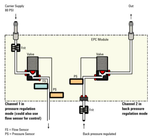
pressure mode can be very useful with a gas sampling valve, where it ensures that the sample pressure in the loop remains constant.
