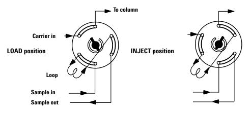
**Load position** The loop is flushed with a stream of the sample gas. The column is flushed with carrier gas.
