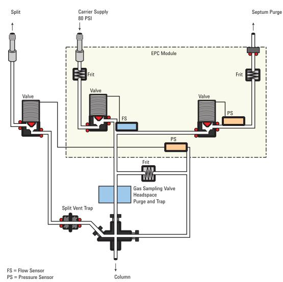
Total flow to the interface is measured by a flow sensor and is divided into two streams. One stream connects to the septum purge regulator; the other connects to a frit block. At the frit block, the flow is further divided. The first stream goes to the gas-phase sampler and from there is introduced into the interface. The second stream, called the pressure sensing line, passes through the frit block and is measured by a pressure sensor. This stream also provides a trickle flow to the interface.
