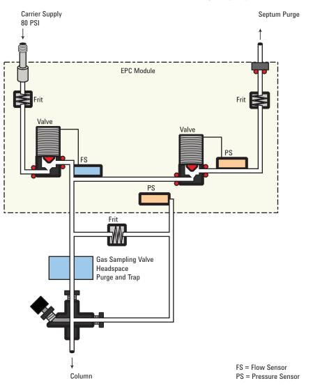
Flow to the interface is measured by a flow sensor and controlled by a proportional valve.
