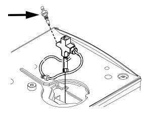
7 Place the interface in the heater block. Replace the clamping plate you removed earlier and tighten the screw until snug. Do not overtighten. If you removed the transfer line, replace it.
