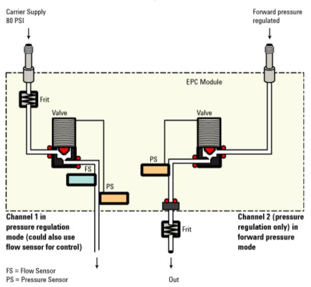
Channel 2 may be used either as a forward-pressure regulator or as a back-pressure regulator, simply by reversing the input and output connections. The back
