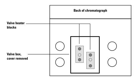
Figure 3 Diagram of valve locations on GC
