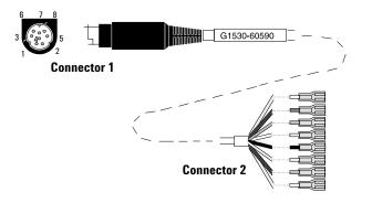
The external event cable (G1530-60590) has two passive relay contact closures with two 24-volt control outputs. Devices connected to the passive contact closures must be connected to their own power sources.
