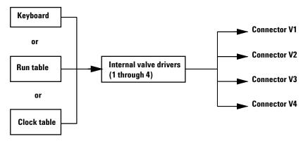
There is no direct relationship between the location of a valve in the valve box and the driver that controls it. This depends on how the solenoids are wired and the actuators are plumbed.
