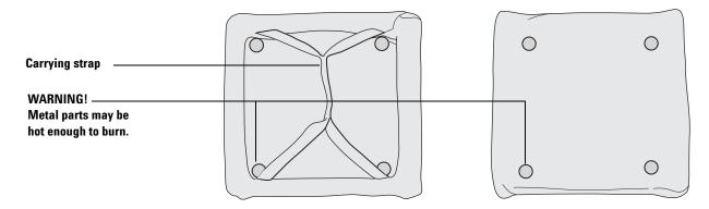
The oven insert is used with any inlet, column, and detector mounted in the **back** position. It is not compatible with any accessory which obstructs access to the front of the oven or which requires the use of either the front inlet or the front part of the oven.
