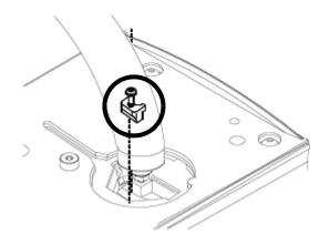
4 Carefully lift the interface out of the heater block.
