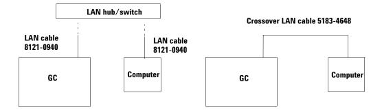
**Figure 4** Connecting the GC and computer with a hub/switch (shown at left) or a crossover cable (shown at right).
