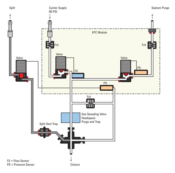
During this user-specified sampling period, the solenoid valve is closed. Flow to the interface is measured by a flow sensor and controlled by a proportional valve.
