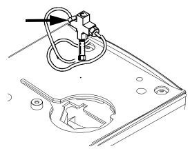
6 Install a blanking nut into the split line port and finger-tighten the nut. Tighten the nut an additional 1/4-turn using two wrenches in opposition.
