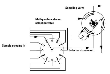
If the GC has one valve configured as a multiposition valve and another configured as a gas or liquid sampling valve, it assumes that they are to be used in series. This "double configuration" can be used to replace an automatic liquid sampler and sample tray in an analytical sequence. The multiposition valve becomes the sample tray; the sampling valve becomes the injector.
