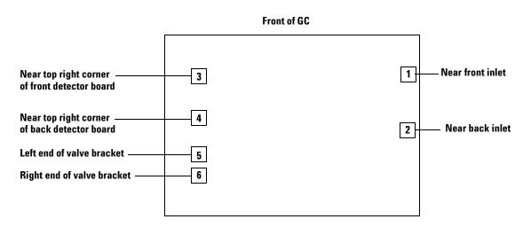
All heater connectors are square, 4-conductor receptacles mounted on brackets.
