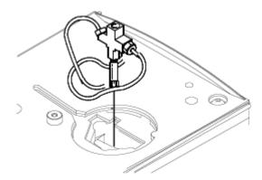
5 Loosen the hex nut connecting the split vent line to the interface until you can remove the line. Put the line aside. You do not need to plug it.
