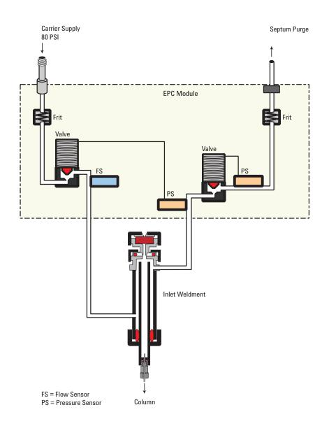
The next figure shows the flow diagram for the packed column mode, with the column not defined the control is based on total carrier gas flow.
