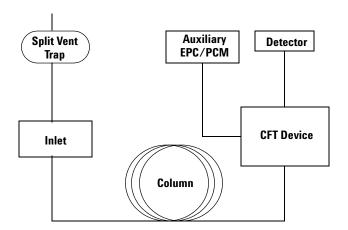
After the last analyte of interest elutes, you can program a decrease in inlet column flow with an increase in the pressure/flow from the Aux EPC or PCM connected to the CFT device, thereby reversing column flow and forcing the remaining analytes off the column and out of the inlet split vent. You can do this using a post run program or as a ramped pressure or flow program.
