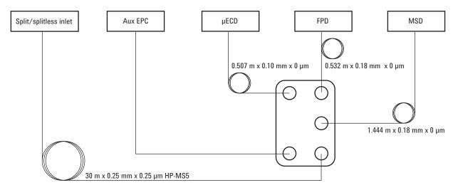
In this configuration, the gas eluting from the column is divided among three detectors. Because the resulting flows can be quite small, makeup gas is added at the splitter. An Aux EPC channel provides it.
