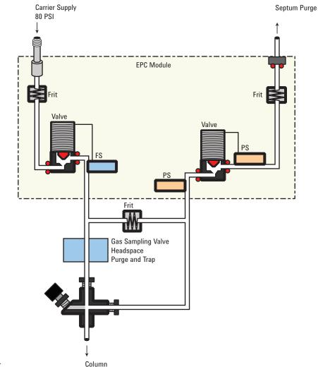
FS = Flow Sensor PS = Pressure Sensor
